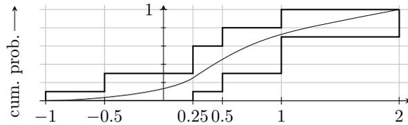
DSIs represent *uncertain* distributions, that is, the set of focal elements in general represents not a single exact distribution, but a set of distributions. Thus DSIs allow us to efficiently and soundly represent the continuous distribution such that the true distribution(s) are guaranteed to be inside the computed DSI. Naturally, the abstraction comes at a cost of certain over-approximations.
